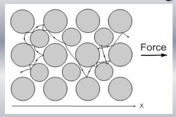
Electrons move between ions in a metal subject to a voltage difference (electric field)
